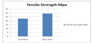
Fig 3. Tensile strength of Sisal/Glass fibre composites
