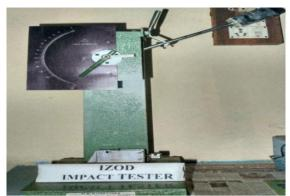
Fig 2. Izod Impact testing machine.
