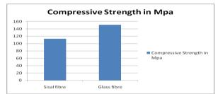
Fig 4. Compressive strength of Sisal/Glass fibre composites
